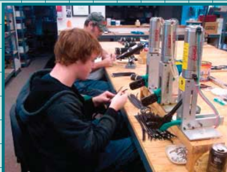
Pneumatic assisted hand tool cylinders insure consistent precise crimps.
